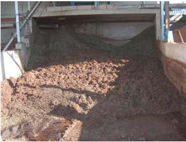
Fig. 1 Wet olive mill sludge (OMS) generated in massive quantities by olive-oil extraction in the olive oil mill
